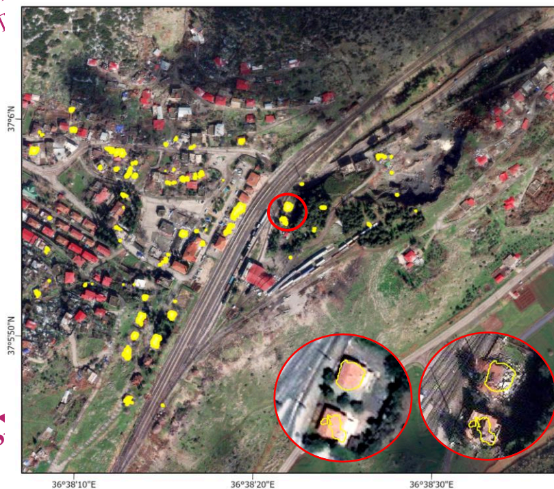
(a) Fevaipasa(底图为震后WorldView影像,黄框标注为SWSACNet识别的倒塌建筑物) (a) Model inference results of Fevaipasa(base map provided by WorldView, yellow marker represents collapsed buildings extracted by SWSACNet)
